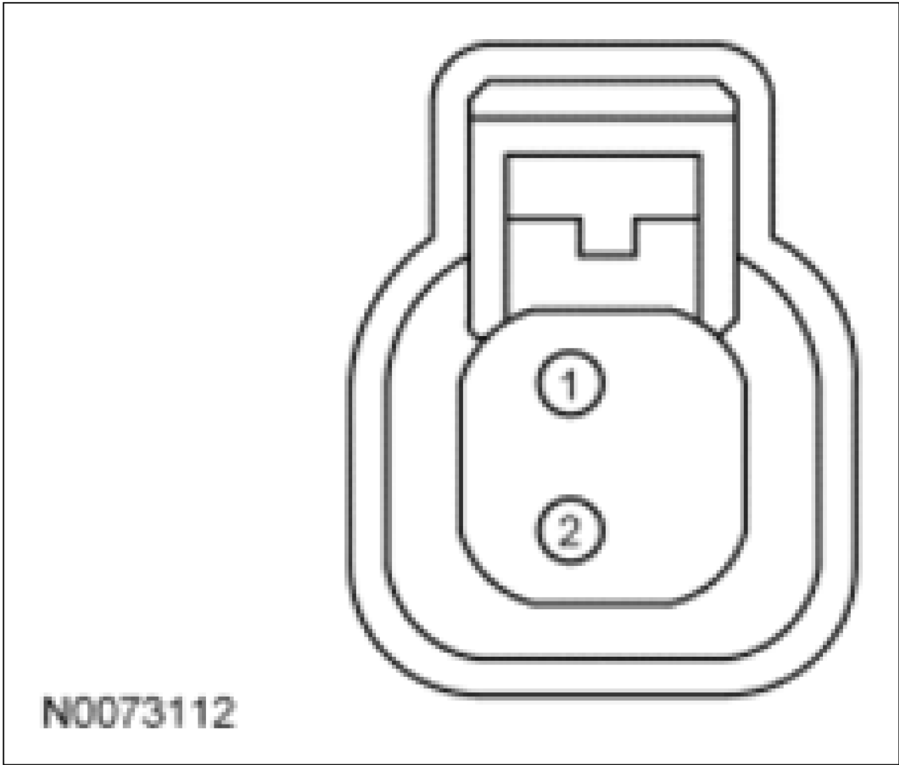
Fig 3: Identifying Cylinder Head Temperature 2 Sensor Connector Terminals
