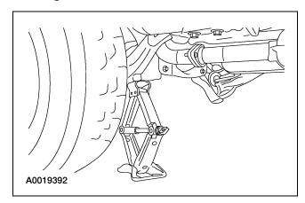
The rear jacking points are located on the rear trailing arms.
