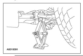
1. The front jacking point is at the bolt head of the lower control arm.
