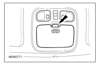
6. **NOTE:** The overhead console is also supported by a retaining clip.
